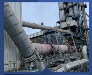
Before the implementation at CEMMAC Cement Plant in Horne Srnie, Slovakia, we measured the temperature of the flue gas chimney surface at 160°C. The chimney posed a danger to employees due to burns, and nearby technologies were affected over time due to an extraordinary heat leak produced by the flue gas chimney. To prevent these issues, we decided to address the situation with the Bronya Classic thermal insulation coating.
