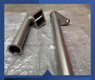
Before commencement, we had to prepare the dry ice conveyor for thermal insulation application, i.e., wrap the parts that didn't require insulation. We used Bronya Antikor and Bronya Classic materials for our client, Rataj a.s. The challenge involved condensation, which couldn't be addressed with conventional insulation due to its inability to prevent condensation. Additionally, standard insulation posed a risk of burns to employees at operational temperatures of -80°C.
